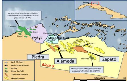
Figure 5.3 – Block 9 PSC with high graded drilling targets
