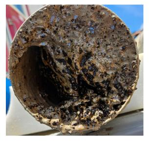
Figure 2 - Core showing the presence of black oil in naturally fractured limestone
