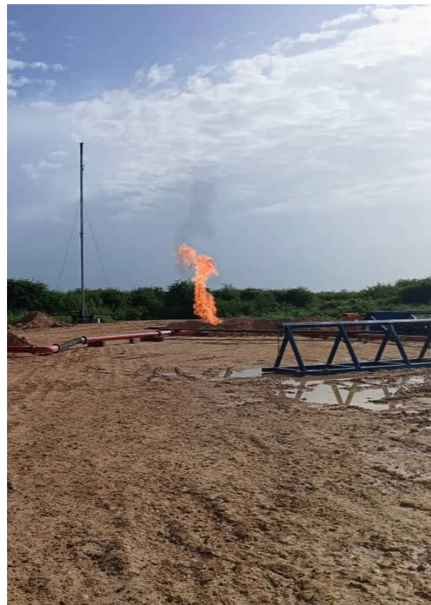
Figure 3 – Testing of oil from Unit 1B in the Amistad interval (sampling and flaring)
