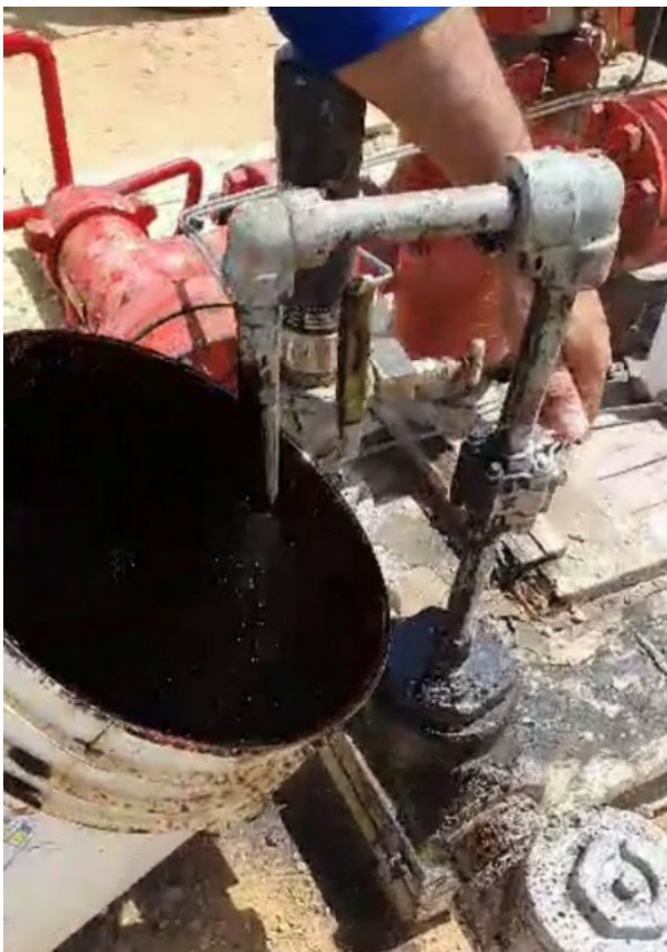
Figure 3 – Testing of oil from Unit 1B in the Amistad interval (sampling and flaring)
