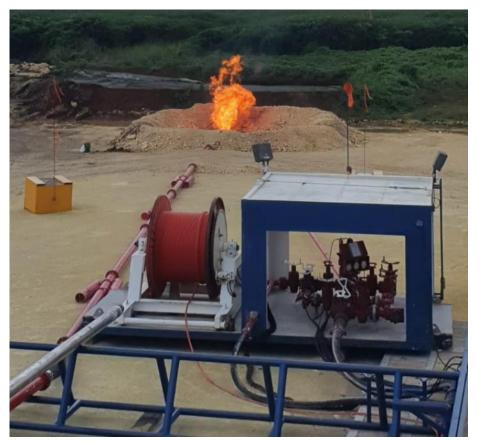
Figure 1 - Flaring of hydrocarbons encountered in the high pressure zone commencing at 1,842 metres
