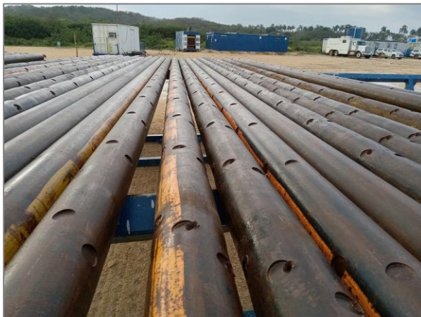
Tubing Conveyed Perforation (TCP) carrier pipe after perforating job.
