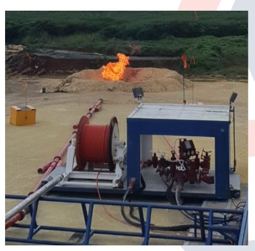
Flaring operations whilst drilling Alameda-1 - Block 9, Cuba
