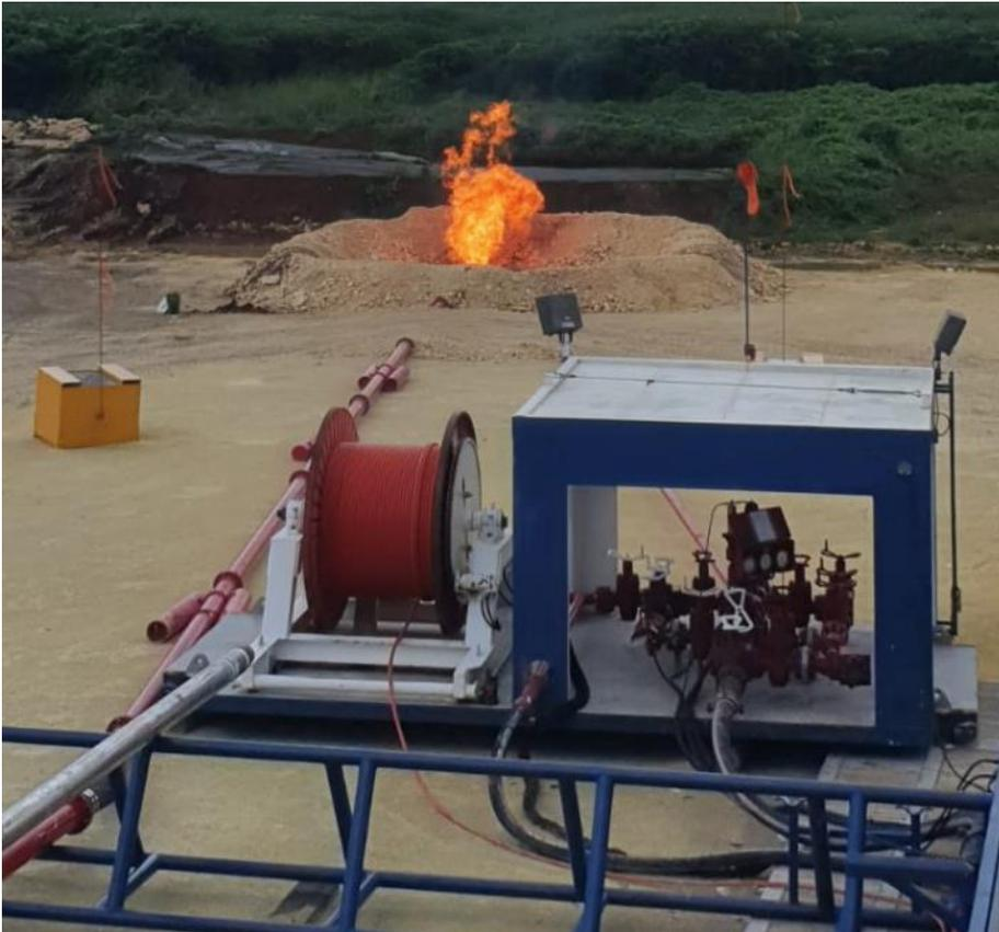
*Figure 1 - Flaring of hydrocarbons encountered in the high pressure zone commencing at 1,842 metres*
