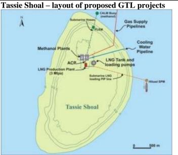
Note: water depth contours are in 20m increments. Water depth where infrastructure is planned is sub-15m. LNG plant uses sea-water cooling substantially reducing the footprint required for an LNG facility.
