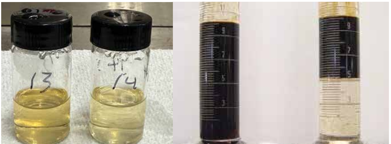
Figure 3 – Melbana RDF (Sample 14, LHS) was designed to maximise production well flows by minimising the risk of formation from crystallisation of precipitates, excessive barite and emulsion formation
