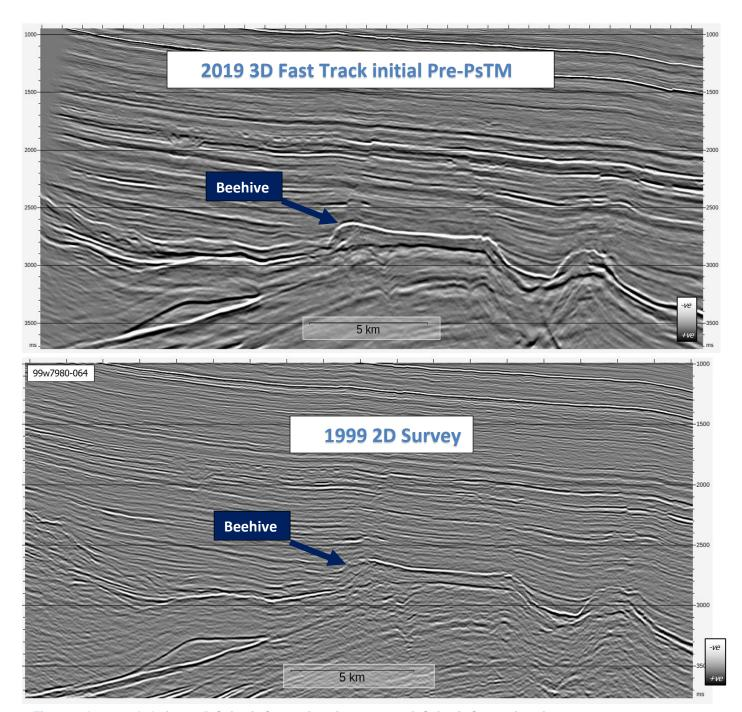
Figure 2: Improved clarity - 3D Seismic Survey imaging vs 1999 2D Seismic Survey imaging
