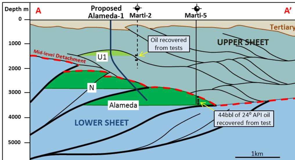
**Figure 2. Schematic cross section for proposed Alameda-1 well**
