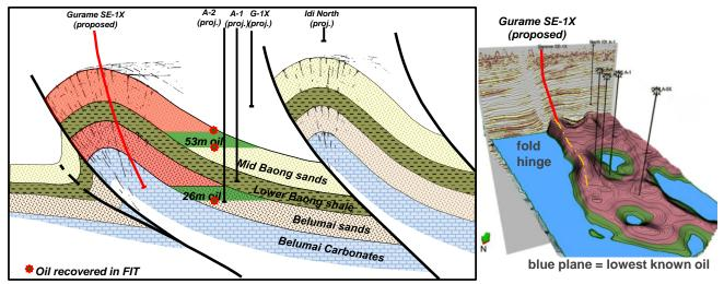
Figure 1. – Simplified Structural Cross Section
