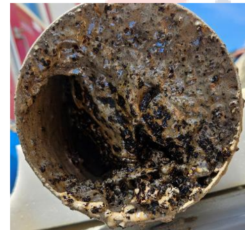
Core from Unit 1A showing the presence of black oil in naturally fractured limestone
