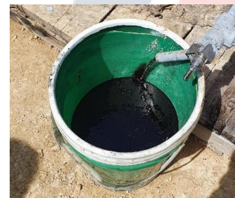
Sampling oil recovered at surface from Unit 1A for lab analysis
