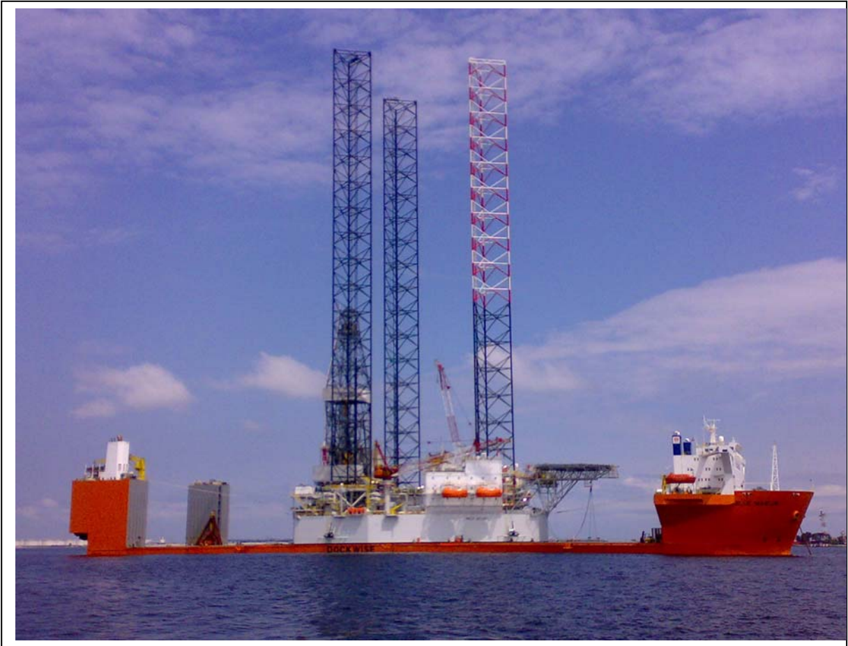
West Atlas Jack-up rig loaded onto the Blue Marlin in Singapore harbour
