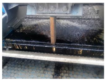
Figure 3 - Free oil on shakers (Zapato-1)
