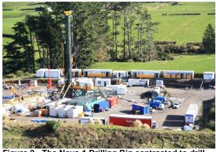
Figure 2 - The Nova-1 Drilling Rig contracted to drill the Pukatea-1 wildcat exploration well
