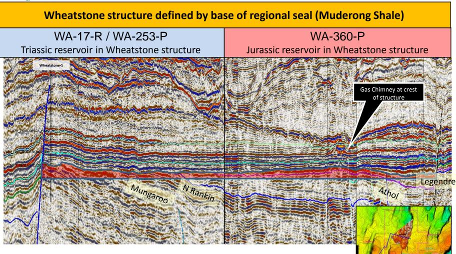
\* Composite 2D and 3D seismic line flattened on Wheatstone GWC
