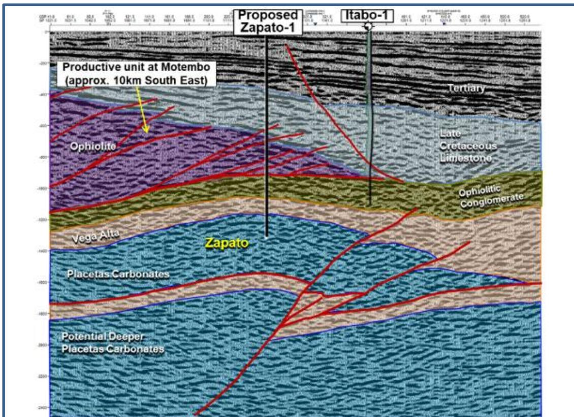
Figure 2 – Zapato Prospect Seismic Profile and Well Path
