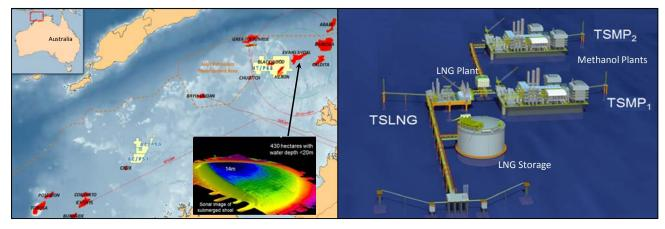
The methanol projects offer the opportunity to develop two 1.75 Mtpa methanol plants based on Davy Process M5000 technology with the potential to accept gas with a  $CO_2$  content of up to 30%. The developments have the potential to provide a commercially attractive development path for the large nearby undeveloped gas resources.
