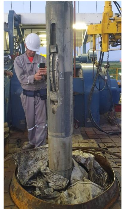
*Figure 1 - Inspecting the underreamer at Alameda-1*
